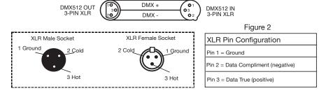
**Special Note:** Line Termination. When longer runs of cable are used, you may need to use a terminator on the last unit to avoid erratic behavior. A terminator is a 90-120 ohm 1/4 watt resistor which is connected between pins 2 and 3 of a male XLR connector (DATA + and DATA -). This unit is inserted in the female XLR connector of the last unit in your daisy chain to terminate the line. Using a cable terminator (ADJ part number Z-DMX/T) will decrease the possibilities of erratic behavior.
