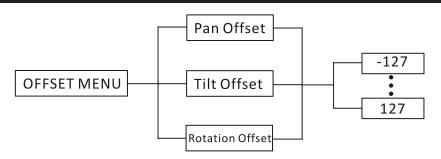
To enter the home adjustment submenu, press the ENTER button for at least 5 seconds. In this submenu you are able to adjust the original position (home position) of certain functions.
